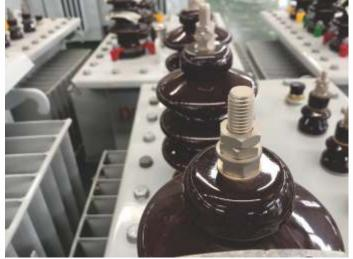
M-Tech manufactures oil immersed transformers with cooling mode ONAN and ONAF as per International Standards IEC 60076, BS 171, VDE 0532, ANSI C 57:12 etc.
